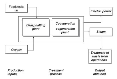
FIGURE C1-1 Graphic Model of the Cogeneration Process
