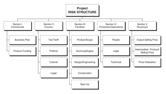
FIGURE 8-3 The Risk Breakdown Structure (RBS): the IPRA model
