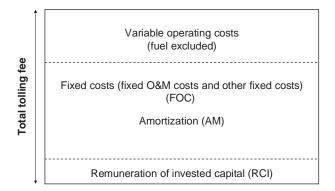
FIGURE 3-12 Structure of the Tolling Fee in the Industrial Approach
