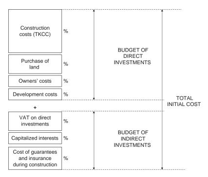
FIGURE 5-3 Items Included in the Construction Cost
