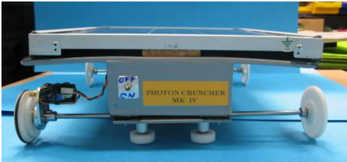
PHOTON CRUNCHER MK IV REAR VIEW Note: The drive wheel (left hand side) is the plastic version with an O ring tyre not the Aluminium drive wheel the test results are for.
