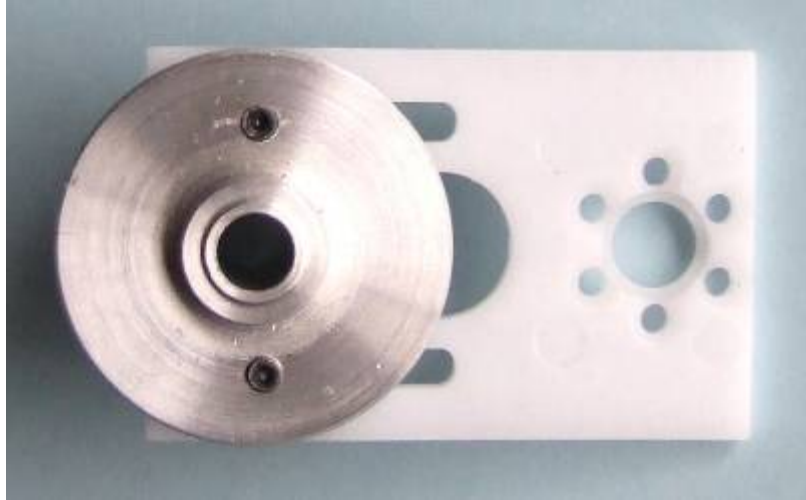
MOTOR MOUNT PLATE AND MOTOR MOUNT FLANGE ASSEMBLY WHEEL SIDE VIEW
