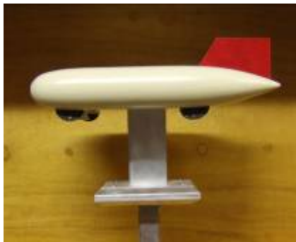
Stretched airship shape (Frontal area 7016 mm sq.)
