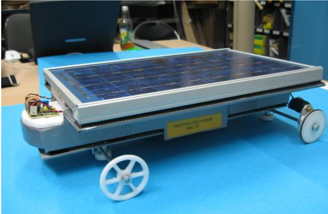
PHOTON CRUNCHER MK IV SIDE VIEW WITH STANDARD DRIVE WHEEL FITTED WITH “O” RING TYRE Note : the Engelec Electronics is mounted in the cockpit so it is visible
