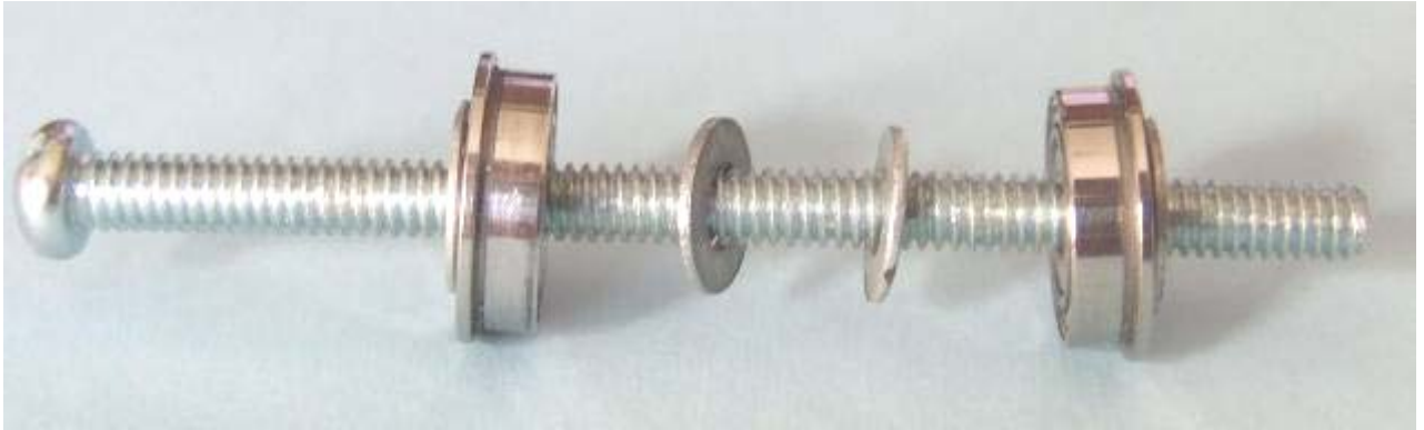
SLEEVES ASSEMBLED INTO BEARINGS
