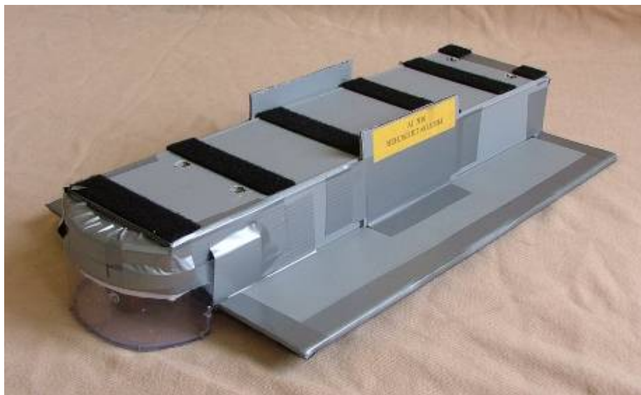
UNDERSIDE VIEW OF BODY (FOLDED CORFLUTE) SHOWING VELCRO USED FOR FIXING BODY TO CHASSIS NOTE: BODY IS ONLY REMOVABLE FOR DEMONSTRATION PURPOSES AT WORKSHOPS
