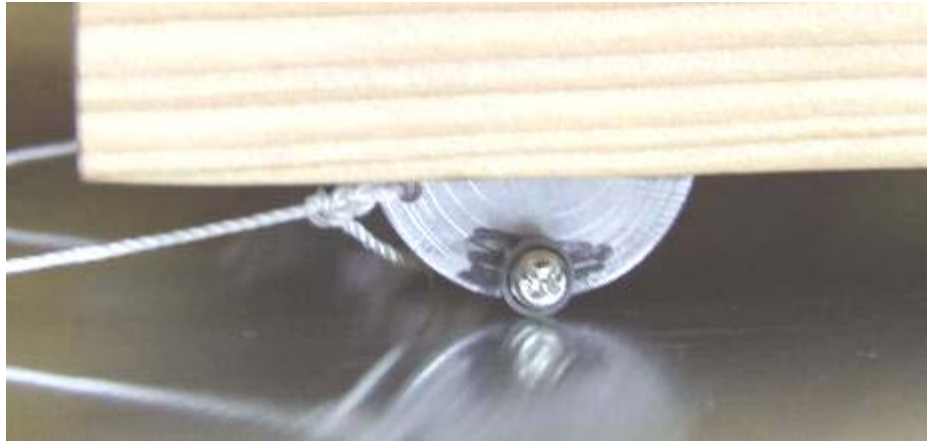
Detail of bearing fitted to wheel
