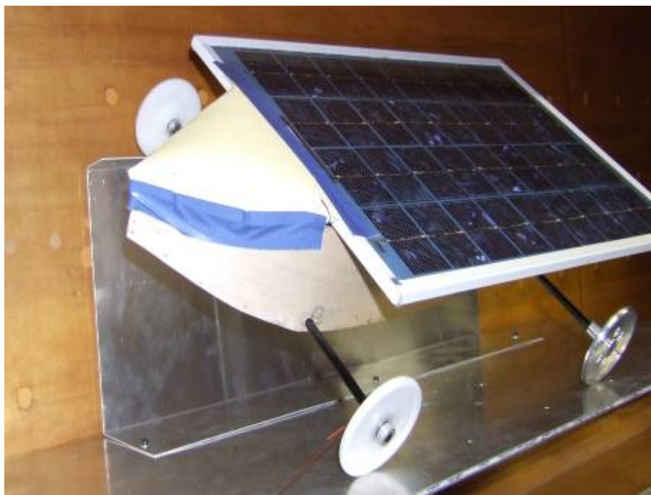
SYNDAL SOUTH 2006 CAR : SIMULATOR AIR DRAG COEFFICIENT 0.0045
