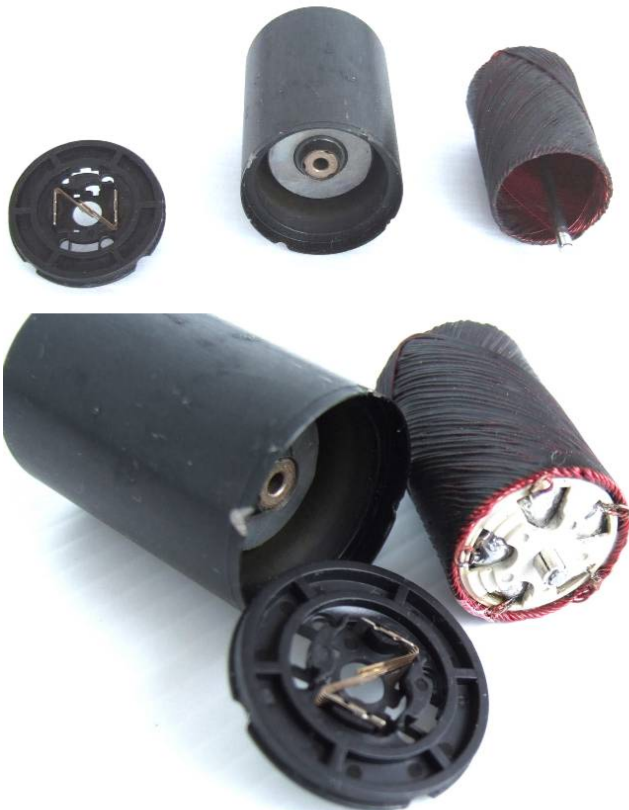
FAULHABER 2232 MOTOR DISASSEMBLED
