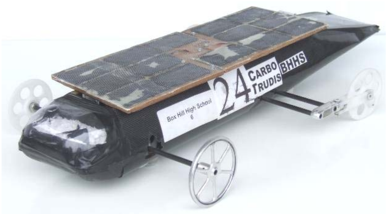
CARBO TRUDIS: SIMULATOR AIR DRAG COEFFICIENT 0.0039
