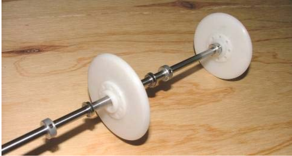
FRONT AXLE DETAIL EXPLODED VIEW OF WHEEL ASSEMBLY SHOWING BEARINGS AND RETAINING BUSHES
