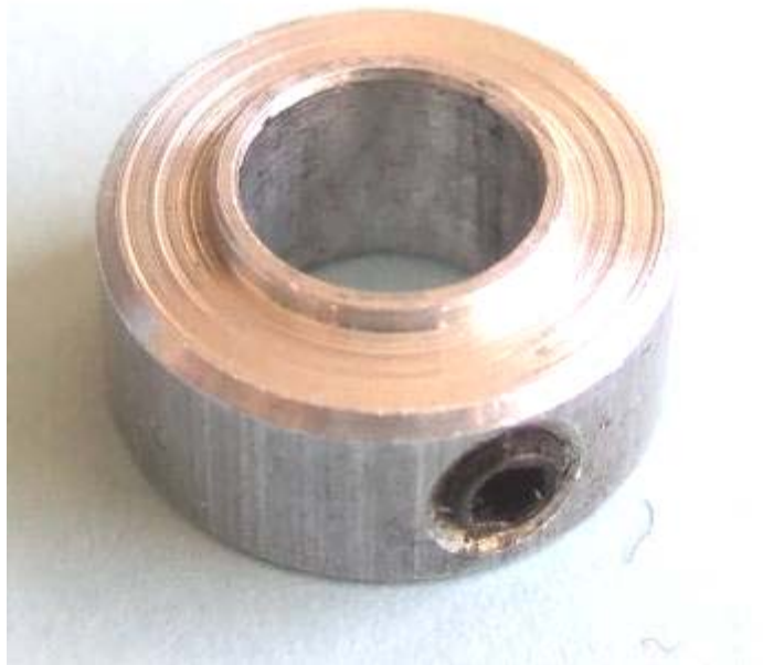
RETAINING BUSH 6MM BORE SCCR06 THE SMALL LIP IS ASSEMBLED FACING THE BEARING
