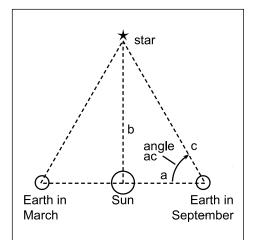
Using parallax to determine the distance to a star is done by calculating the apparent shift of a star as the Earth orbits the Sun.
