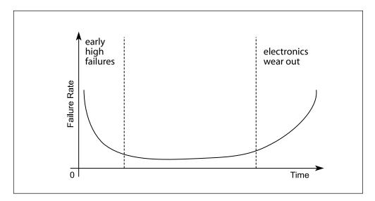
Calculations involving the common failure rates of various mechanical devices often results in a graph with a bathtub-shaped curve.
