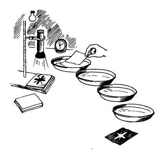
caused the silver to separate from the silver chloride in the exposed areas, and since the silver is dark, those areas became dark. The solutions that you later dipped the paper into caused the remaining silver chloride to dissolve and transformed the pure silver into an insoluble silver salt that won't wash away.
