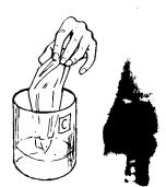
Results: The color disappeared from the cloth. The reaction between the calcium chlorate and nitric acid produced hypochlorous acid (HClO), which in turn caused the bleaching. The equation for this reaction is:
