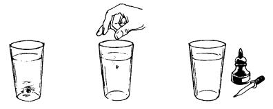
Results: At first the potassium permanganate crystal made a thin line of color as it fell through the water. Soon the water around the crystal became colored. After standing all night, the crystal dissolved almost completely and the entire glass of water became the same shade of violet.
