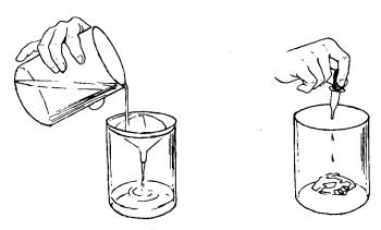
fifth jar. CAUTION: Do not let any of the acid touch you. Clean the eye dropper and use it to squirt with even pressure the blue solution from the fourth jar into the jar of dilute sulfuric acid. Hold the tip of the dropper under the surface of the sulfuric acid. Finally, remove the result with the glass stirring rod and wash and dry it.
