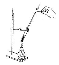
Results: When you heated the coal, it gave off the gases, mainly methane  $(CH_4)$  and ethane  $(C_2H_6)$ , that were trapped in it as it was formed in the earth. This gaseous mixture burned with a characteristic blue flame. The material which remained in the test tube is a form of carbon called *coke*. If there was any sticky brownish substance there, too, it was a combination of *coal tar* products, which are the residue of coal burned in this way.
