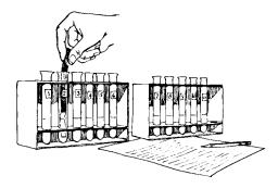
Results: The carbonic acid, the hypochlorous acid, the boric acid, and the acetylsalicylic acid turned the blue litmus paper to red, but had no effect on the red litmus paper. The sodium hydroxide and the ammonium hydroxide turned the red litmus paper to blue, but had no effect on the blue litmus paper. The sodium chloride, magnesium sulfate, ethanol, salad oil, and sodium bicarbonate had no effect on either the red or blue litmus paper.
