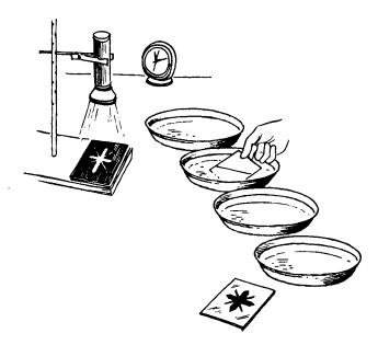
Repeat this procedure with each of the photographic plates. You may find that varying time intervals and different thicknesses of the gelatin coating produce more or less successful results. You will want to experiment a bit until you find the best time exposure for the plates you have made.
