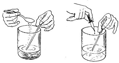
stirring the solution all the time. If the solution becomes dark blue, you will have to start all over again. When the ammonium hydroxide ceases to make the solution turn any lighter, pour the liquid through a funnel lined with filter paper into the third jar. Now put the filter paper and everything caught in it into the fourth jar. Add just enough concentrated ammonium hydroxide to dissolve the filter paper. Pour 11 tablespoonfuls of dilute sulfuric acid into the
