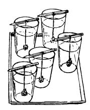
the same shape and had the same general appearance regardless of size. Crystals tied on the string were *seed* crystals. They provided surfaces for the others to grow around. When the solutions cooled, some of the solute separated out in crystalline patterns, characteristic of the particular solute.
