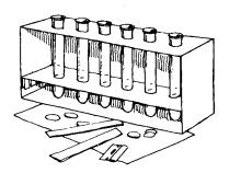
bottom. Slip an empty test tube into each hole in the top and through the hole directly below it. If you traced the holes correctly, the tubes will fit. Cover the surfaces of your test tube rack with aluminum foil to make it last longer. You will need several of these racks, and you will want to replace them as soon as they become wet or contaminated with chemicals. If you have test tubes of more than one size, you will have to find different boxes to fit the various sizes.
