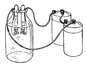
Attach one end of a 4-inch piece of copper wire to the outside terminal of the same dry cell.
