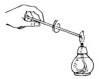
and repeat the process on the other end. CAUTION: If you keep the glass in the flame for too long, it will melt, the hole will close, and you will have a closed tube instead of an open one.
