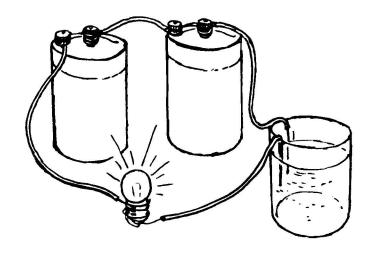
dry cell. You now have this arrangement from left to right: 6-inch wire, dry cell, 4-inch wire, dry cell, 6-inch wire. Wrap one of the loose ends of wire around the threads (screw-type grooves) of the flashlight bulb. Be sure the connection is very tight. In the remaining wire, make an S-shaped bend about 2 inches from one end, so that you can rest it on the edge of a jar. Make a similar S-shaped loop in the free end of the wire connected to the dry cell. Check the diagram.
