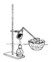
Allow most of the liquid to boil away. Note the color of the liquid collected in the jar.
