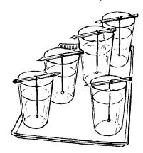
in, move them to a slightly cooler place. Move the whole tray at once and do it gently, so that the contents of each glass remain undisturbed. After an hour, move them to a still cooler place, perhaps the refrigerator. Lowering the temperature gradually and moving the tray without disturbing the contents of the glasses is extremely important for the success of this experiment. Once the solutions have cooled to about 40° F., let them stand for several days.
