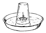
in proportion to the difference in pressure. This gives you a mathematical way of measuring the amount of oxygen used up. Since all the oxygen originally contained in the air inside the glass was used up, what you are calculating is the proportion of oxygen originally contained in that air.
