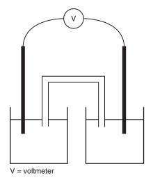
The above galvanic cell is constructed with a cadmium electrode in a 1.0 M  $Cd(NO_3)_2$  solution in the left compartment, and a silver electrode in a 1.0 M  $AgNO_3$  solution in the right compartment. The salt bridge contains a  $KNO_3$  solution. The cell voltage is positive.
