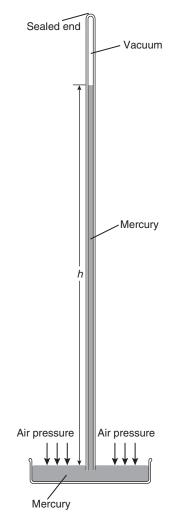
Figure 8.1 The mercury barometer.
