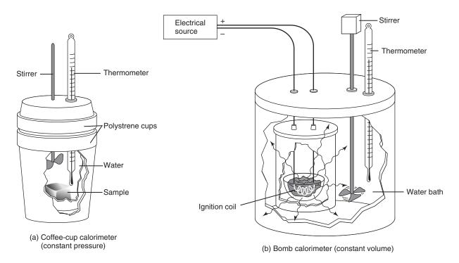
Figure 9.1 Two types of calorimeters.
