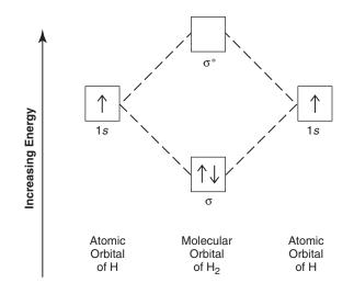
Figure 11.9 Molecular orbital diagram of H<sub>2</sub>.
