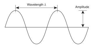
Figure 10.2 Wavelength and amplitude of a wave.
