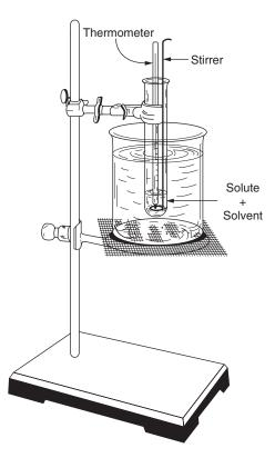
Figure 19.2 Freezing-Point Depression Apparatus.
