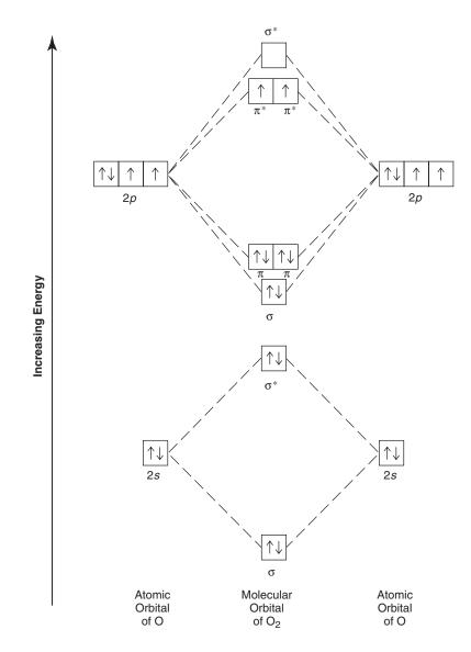
Figure 11.10 Molecular orbital diagram of valence-shell electrons of O<sub>2</sub>.
