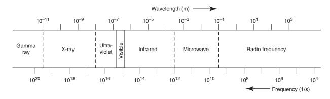
Figure 10.1 The electromagnetic spectrum.
