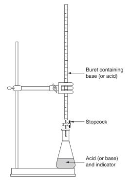
Figure 19.3 General acid-base titration set-up
