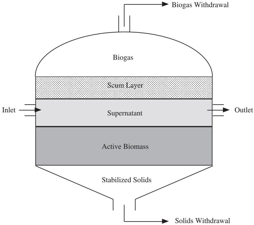
**Figure 1.1** Suspended growth anaerobic digesters are commonly used at municipal wastewater treatment plants for the degradation of primary and secondary sludges. These digesters produce several layers as a result of sludge degradation. These layers are from top to bottom: biogas, scum, supernatant, active biomass or sludge, and stabilized solids.
