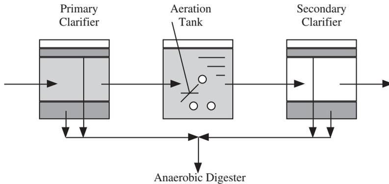
**Figure 1.3** Primary and secondary sludges typically are degraded in suspended growth anaerobic digesters at municipal wastewater treatment plants. The sludges contain relatively large quantities of particulate and colloidal wastes.
