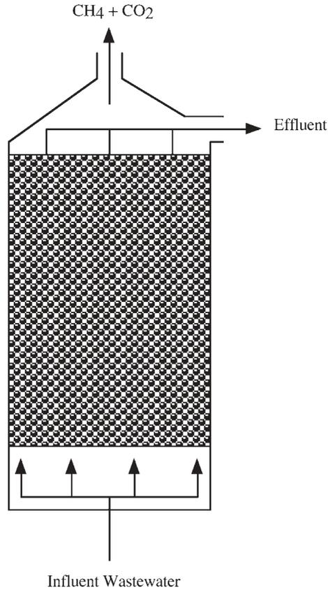
**Figure 1.6** In an anaerobic filter, wastewater flows from bottom to top or top to bottom of the treatment unit. The wastewater passes over media that contains a fixed film of bacteria growth that degrades the organic wastes in the wastewater.
