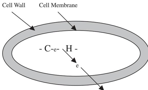
**Figure 3.6** Electrons ( $e$ ) released from broken chemical bonds of substrates inside a bacterial cell are removed through the use of electron transport systems. These systems employ the use of proteins that contain co-enzymes such as metals and vitamins.
