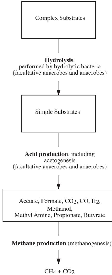
**Figure 7.1** There are three basic stages of the anaerobic digestion process and production of methane. These stages include the solubilization of complex organic compounds or hydrolysis, the production of simplistic acids or acid production, and the formation of methane or methane production.
