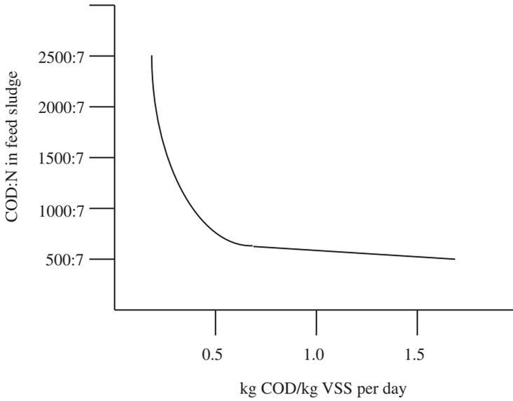
**Figure 15.1** Nutrient needs of an anaerobic digester are determined by the loading or the COD:N and COD:P in the feed sludge. With increasing COD loading there is a corresponding increase in nutrient needs for nitrogen and phosphorus.
