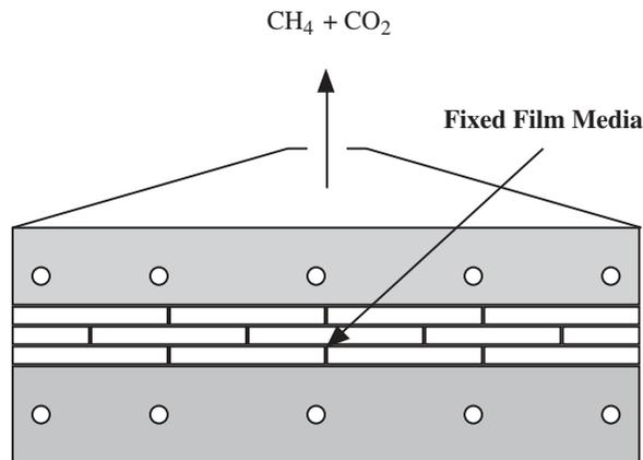
**Figure 1.2** Fixed film anaerobic digesters employ the use of a medium such as plastic or rocks on which bacteria grow as a biofilm. Wastewater passing over the medium is absorbed and adsorbed by the biofilm and degraded.
