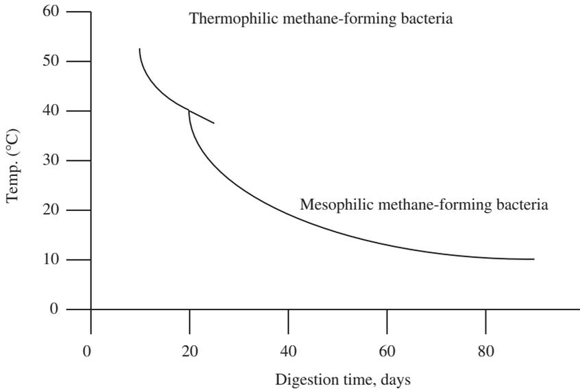
**Figure 14.1** Methane production occurs over a relatively large range of temperature values. Most anaerobic digesters, especially those at municipal wastewater treatment plants, operate in the mesophilic range of temperatures.
