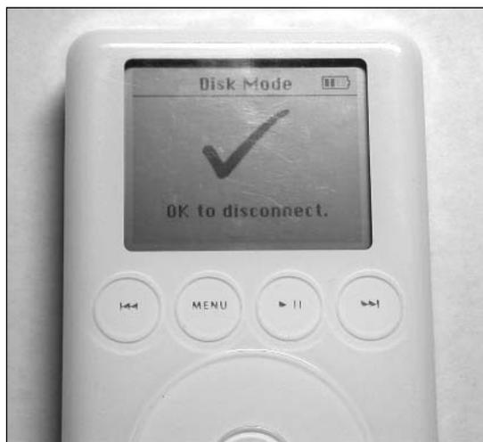
Ryan had temporarily turned the iPod into a disk drive for analysis, and it was time to process the data on the drive. Ryan chose a Mac as an analysis platform, because it could handle both FAT32 and HFS+ filesystems, the default formats for Mac and Windows formatted iPods, respectively. A Windows platform would have trouble processing a Mac-formatted iPod, and Linux was a reasonable choice, but Ryan never could get the HFS+ support working well enough for forensic use. The
