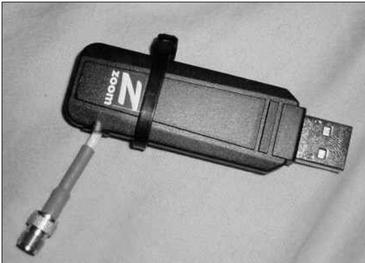
Once I finished the pigtail assembly, I hooked up the yagi to test it out. I'd found a tool named GreenPlaque<sup>1</sup> to scan for Bluetooth enabled devices. Greenplaque<sup>1</sup> was a multi threaded scanner that (unlike the most recent version of White Fang) could scan asynchronously using multiple dongles. Because of this, it scanned multiple channels with better reliability than other tools that I had tested. As
