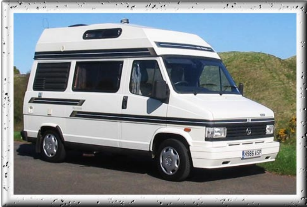
An Autosleeper Harmony Campervan on a Talbot Express base vehicle, 1991. Camper vans are built using a conventional van, to which either a raised roof has been added or had the back replaced by a low-profile body (aka coach-built).
