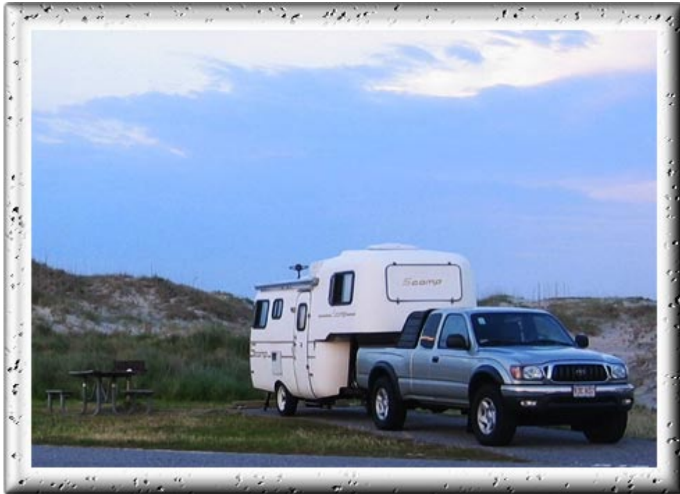
The Outer Banks, NC. 19' Scamp 5th Wheel + 6-cyl Toyota Tacoma. Designed to be towed by a pickup or medium duty truck equipped with a special hitch called a fifth wheel coupling. Part of the trailer body extends over the truck bed, shortening the total length of vehicle plus trailer combined. Some larger fifth-wheel trailers, usually over 40 feet (12.2 m) in length and 18,000 pounds (8,200 kg) in weight, are pulled by small semi-trucks, such as a small Freightliner.
