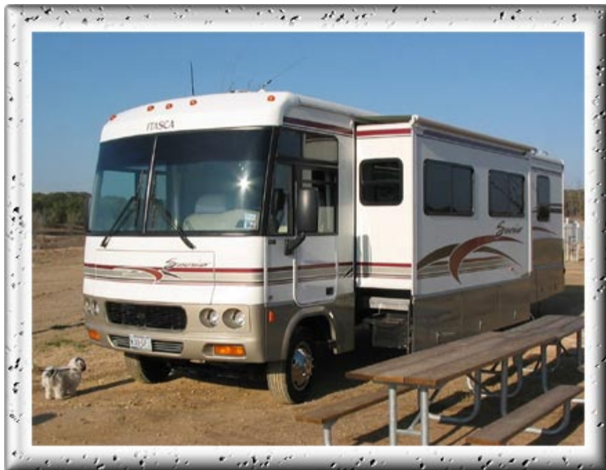
A Class A motorhome with the slide-out extended. And a cute little dog who knows this is HOME! Constructed on either a commercial truck chassis, a specially designed motor vehicle chassis, or a commercial bus chassis. The addition of slide-outs, first appearing in 1989, dramatically changed the industry, as they allow a wider room than would fit on the road.
