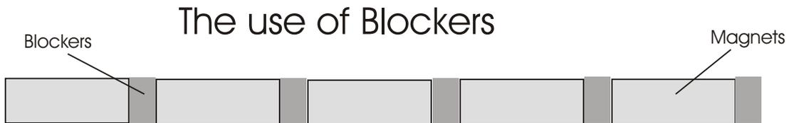
Blockers are iron or steel placed between 2 magnets, the flux field is made alot less stronger and
