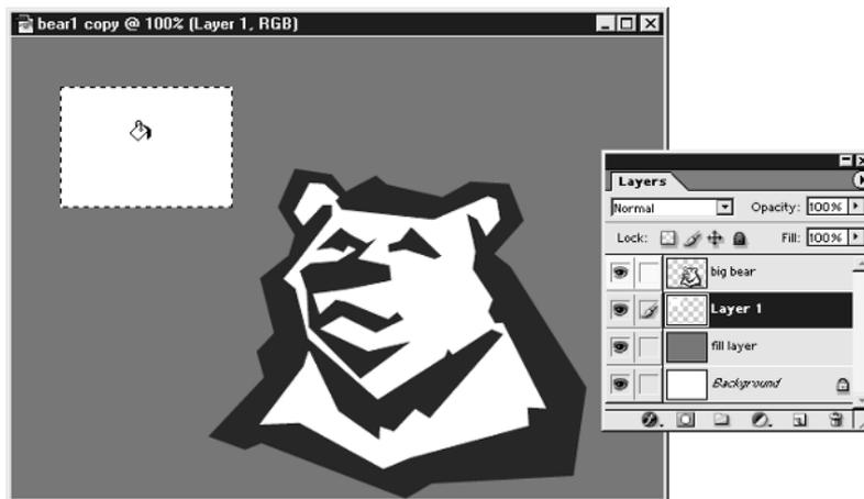
**FIGURE 2-5** An active selection is shown by a dashed line.
