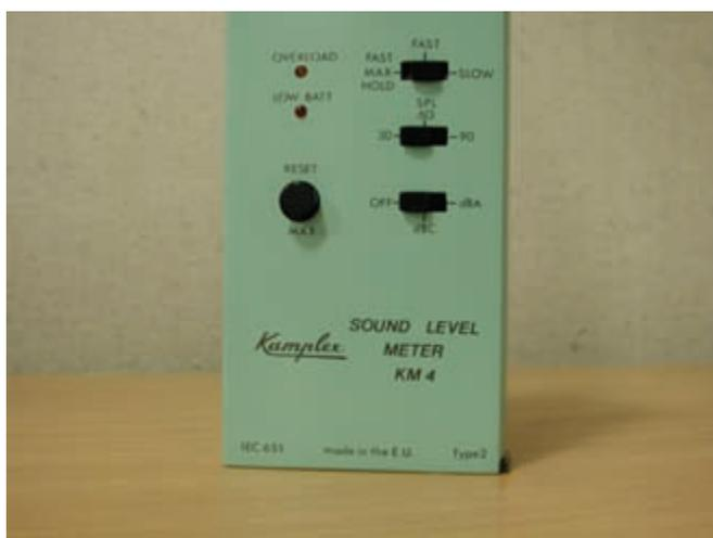
Figure 5.6 Sound pressure meter.
