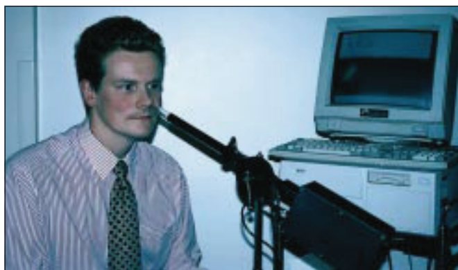
Acoustic rhinometry measures cross sectional areas of the nasal airway
