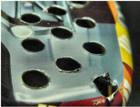
Figure 8-12. Exposed metal on drill holes causes unintended electrical connections
