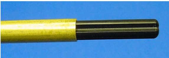
Figure 20-5. LEGO cross axle inserted into \frac{7}{32} -inch diameter tubing
