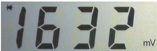
Figure 10-17. Multimeter displaying normal LED value
