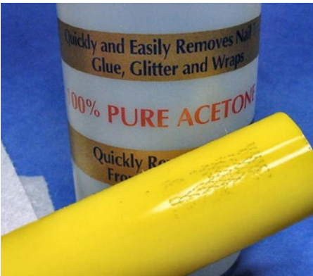
Figure 24-16. Removing sticker adhesive residue with acetone
