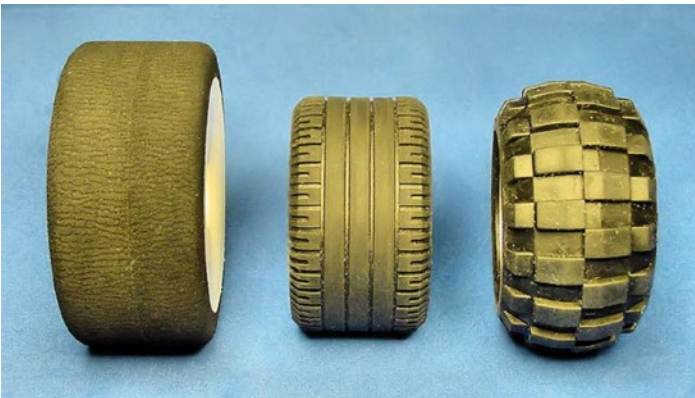
Figure 19-5. Tread designs (left to right): Slick, grooved, and knobby
