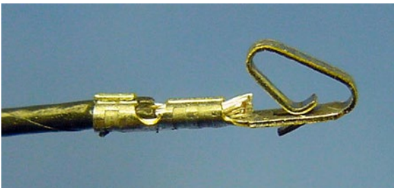
Figure 22-17. Two crimps attaching wire to terminal
