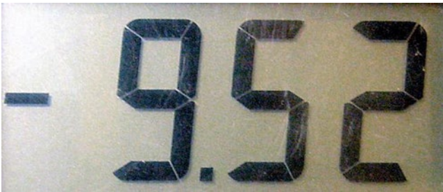
Figure 7-6. A negative number indicates a mixed-up connection
