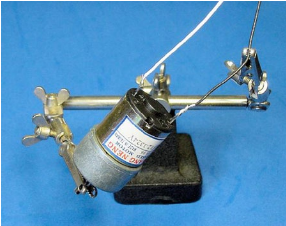
Figure 22-4. Helping hands holding motor and wire in preparation for soldering
