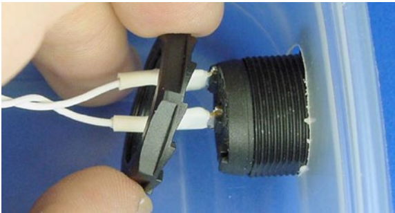
Figure 24-22. Locking nut being screwed onto rear of power switch
