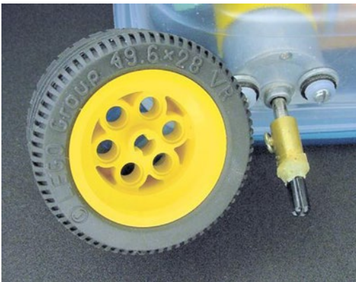
Figure 6-16. LEGO wheel (left) and coupler on motor (right)
