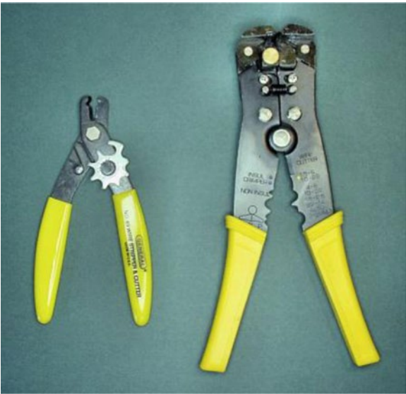
Figure 12-20. Adjustable and automatic wire strippers
