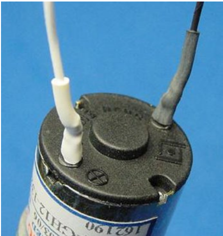
Figure 22-11. Heat-shrink tubing after heating; protecting and insulating soldered terminals
