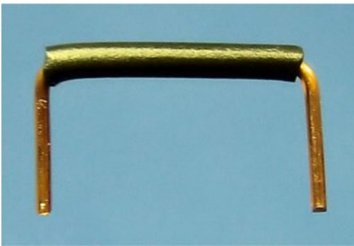
Figure 12-22. Completed homemade flat jumper wire
