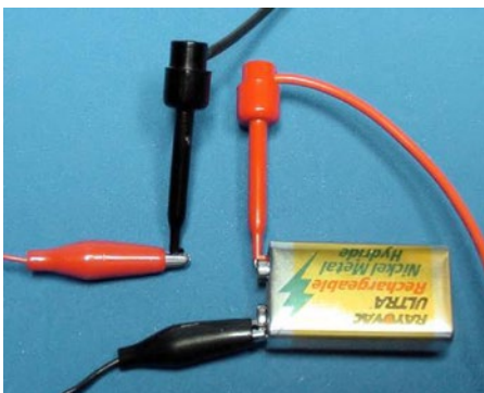
Figure 11-9. Power indicator circuit connection for current-flow measuring
