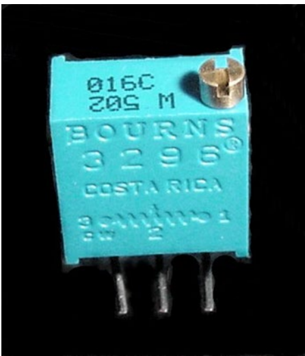
Figure 14-4. A breadboard-compatible multiturn trimpot
