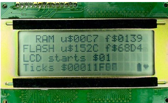
Figure 27-23. Standard 14-pin 20-character by 4-line LCD
