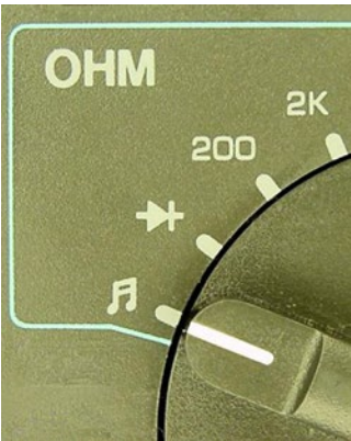
Figure 8-5. Multimeter dial set to continuity
