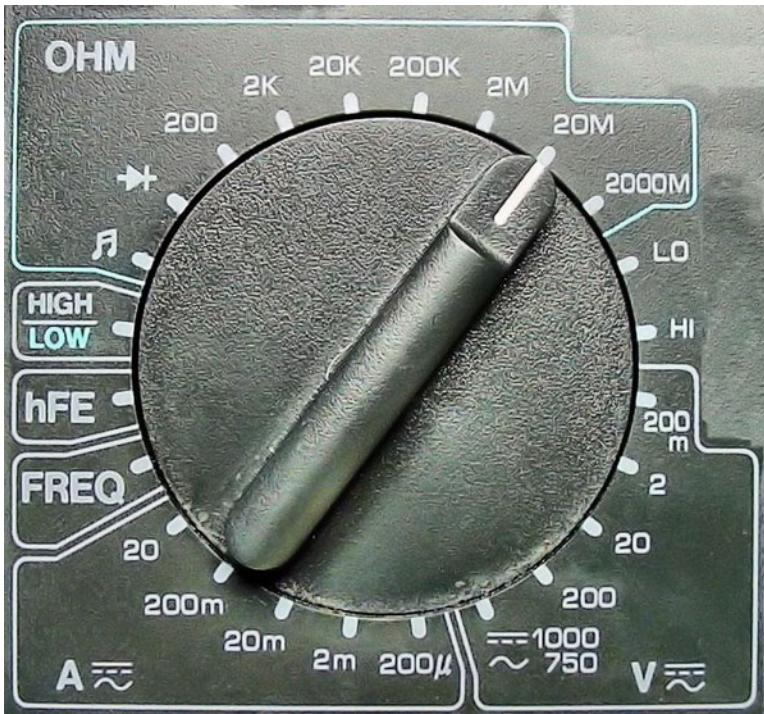
Figure 4-7. Dial with groups of manual range settings
