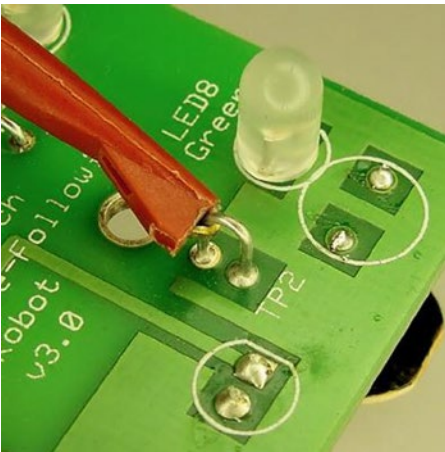
Figure 25-6. A multimeter test lead IC hook firmly grasps a loop of wire for a sensor test point
