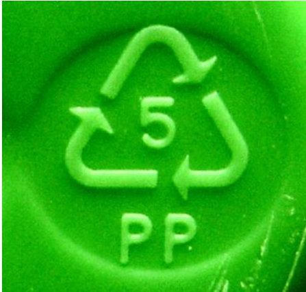
Figure 24-17. Recycling symbol indicates tube is polypropylene
