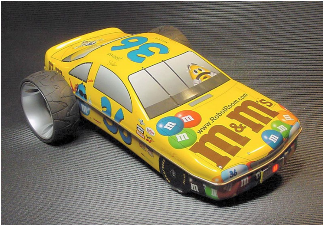
Figure 1-12. Line-following robot made from a candy container
