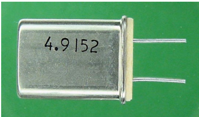
Figure 5-5. Missing multiplier and units (should be 4.9152 MHz)
