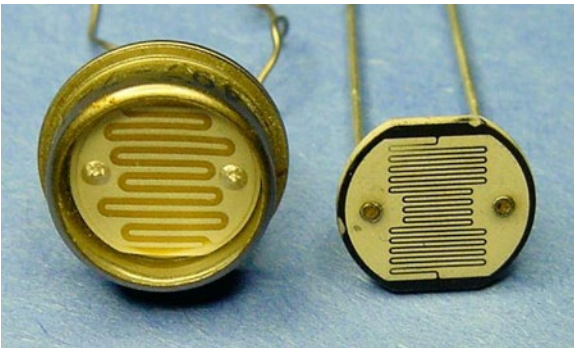
Figure 14-12. Encapsulated and exposed ceramic cadmium-sulfide photoresistors
