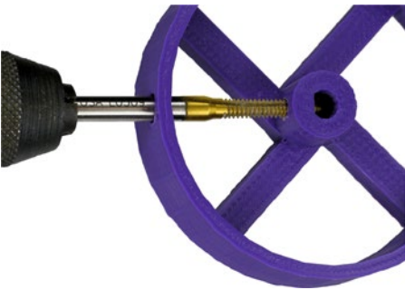
Figure B-15. Tapping set screw threads through a hole in the rim
