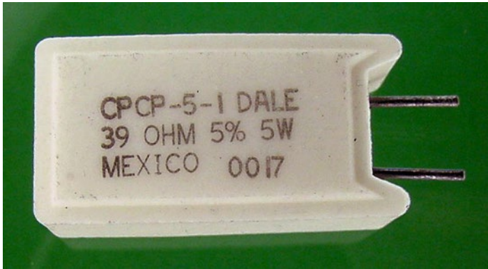
Figure 5-4. A part with plenty of room for a descriptive label
