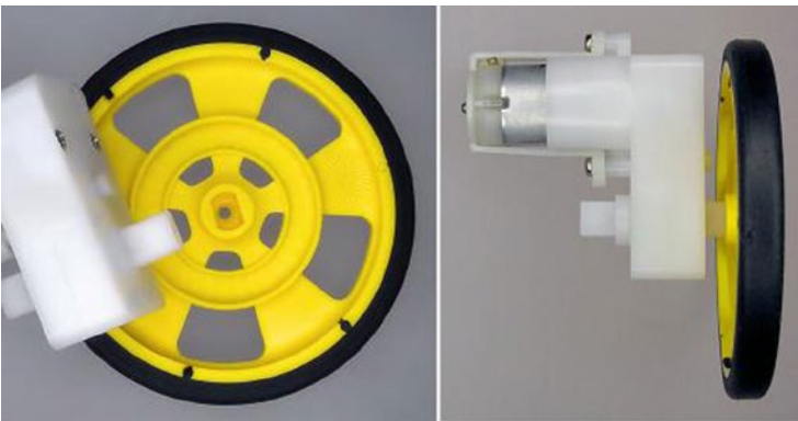
Figure 18-2. Solarbotics GM2 motor with matching wheel
