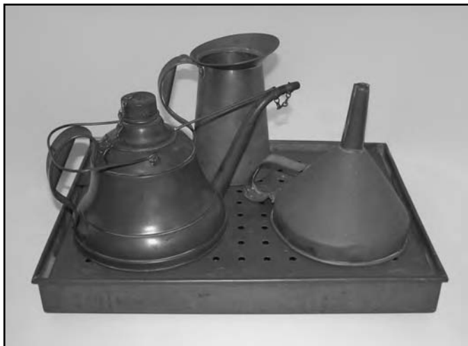
Lighthouse keepers had to polish a lot of brass, including brass tools. These brass items—a lamp oiler, oil measuring pitcher, and funnel—were placed on a drip tray that collected spilled oil for reuse. Michigan Lighthouse Conservancy
