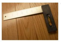
This flat metal ruler bends 90 degrees into a "L' shape. It's helpful for framing up lumber, and doing all kinds of woodworking, especially as a saw guide.
