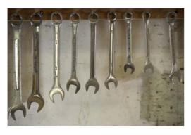
A **crescent wrench** can be very helpful in removing nuts and bolts. It has an adjustable head that fits around the fastener to be unscrewed. The non-adjustable **combination wrenches** are usually sold in sets, as their head openings only fit one size of bolt apiece.
