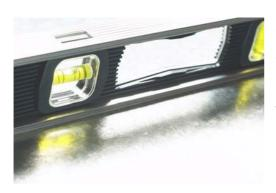
Levels are generally lengths of metal with enclosed capsules of water. When it's placed atop a level object, the bubbles in the water line up with a set of guides. There are many new variations of this basic tool, including electronic models that use lasers.
