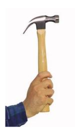
A good hammer is a relatively simple thing to find. Select an 8-ounce, claw-type (for pulling nails) hammer to begin with, and then move onto a more sturdy and efficient 16-ounce model once you get sick of tapping your nails in instead of pounding. A hammer is the linchpin of your toolbox, and, behind the various types of screwdrivers, probably will be the most-used item.
