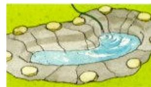
**3. Use a hose to gradually fill the liner with water, weighting the liner with stones around the edge.**
