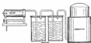
Image Figure 8.--Oxygen from Chlorate of Potash
