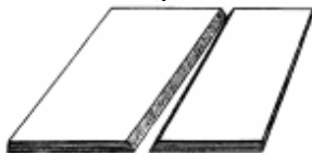
Image Figure 28.--Tapering the Opening Formed by a Break
