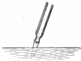
Image Figure 6.--Cooling the Tool for Tempering
