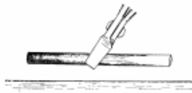
Image Figure 5.--Cooling the Test Bar for Hardening
